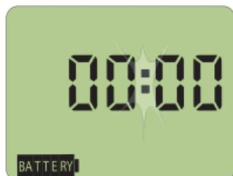
To completely restore the default factory settings press the two arrow Keys ◀ and ▶ for approximately 5 seconds until 00:00 is shown on the display.
