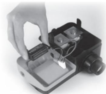
1. Press the two side buttons on the front panel then insert one new 9V Alkaline battery into the terminal.
